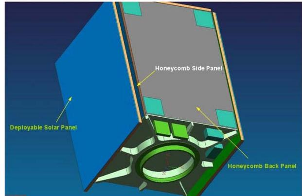
**Fig. 1** X-SAT launch configuration with folded solar panels. The two GPS antennas close to the launch adapter face the -z-axis (zenith during earth-pointing mode).
