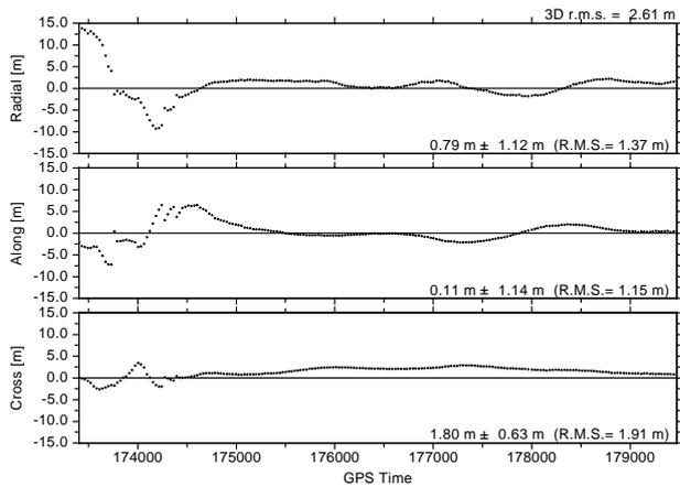
**Fig. 5** Absolute position residuals in the radial, tangential, and normal (RTN) frame with respect to the reference trajectory [17].
