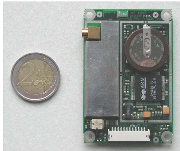
**Fig. 2** Phoenix receiver board
