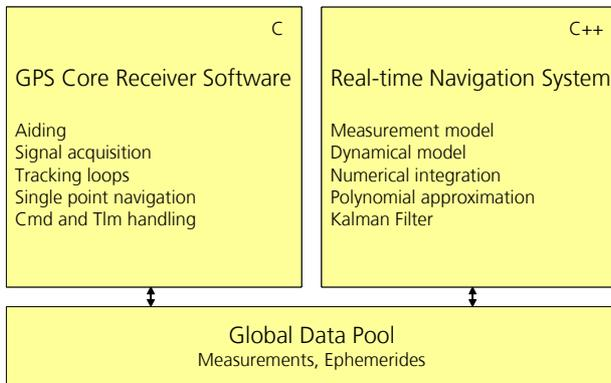
**Fig. 3** XNS basic software architecture
